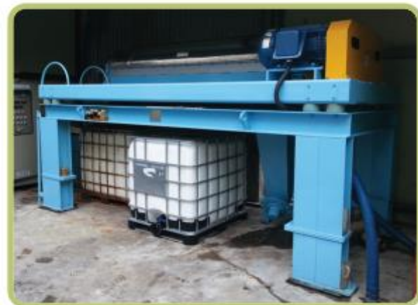
3 Phase Centrifuge Separator
