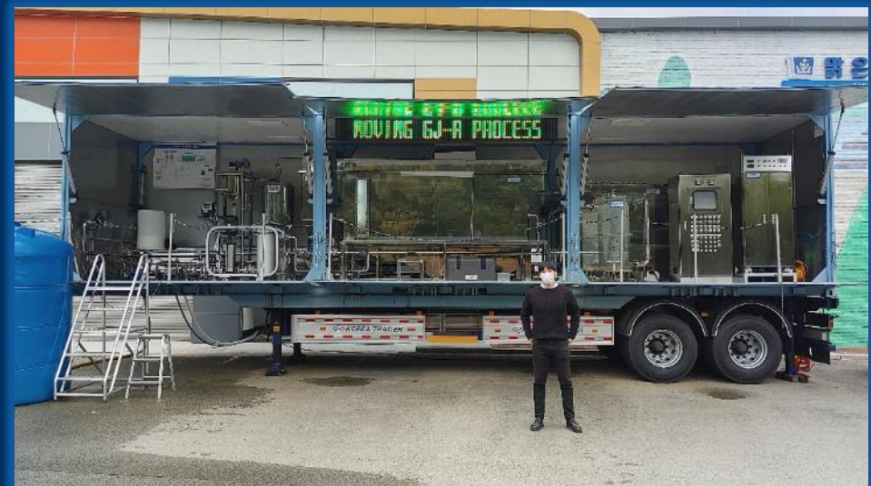
Portable Mobile Skid type 100m 3 /day
