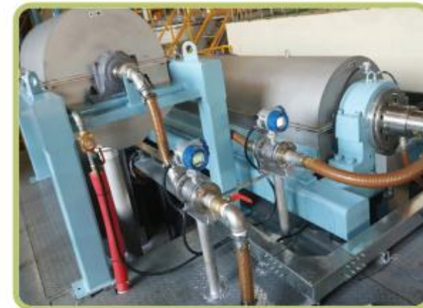
Low speed Solid-Liquid Separator
